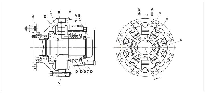
Hydraulic motors of the type MCR-C are radial piston motors with rear case mounting and flanged drive shaft. These motors have a compact front housing and are intended for drives in open or closed circuits. These motors are used in a wide range of applications where there is lower external loading. The integrated flange with wheel studs allows easy installation of standard wheel rims.
