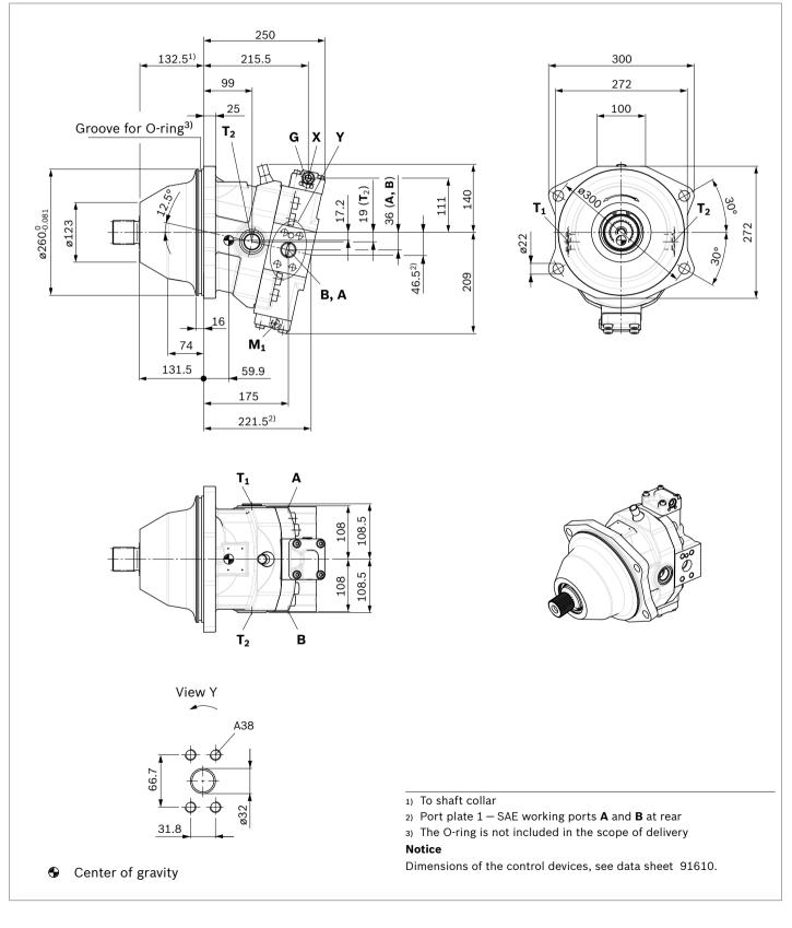
▼ Location of the working ports on the port plates (View Z)
