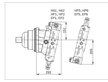
ISO 6149, ports plugged (in normal operation). For notes on tightening torques, see instruction manual. The countersink can be deeper than as specified in the standard.
