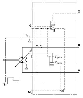
▼ Circuit diagram HZ7 (negative control) size 60 to 115
