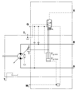
12 **A6VE Series 71** | Variable plug-in motor HP – Proportional hydraulic control
