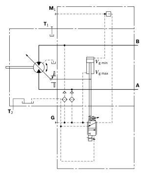
▼ Circuit diagram EP5, EP6 (negative control)
