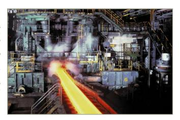
The application conditions supported by the bearings are variable but always very difficult: very high pressures (rolling), high temperatures and heavy loads, humidity (water projection cooled the high temperature parts), vibration and shocks.
