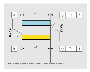
They must be sufficiently rigid to avoid any bending during tightening. Their length should not exceed 200 mm. Their face parallelism tolerance and permissible length variances are specified below.
