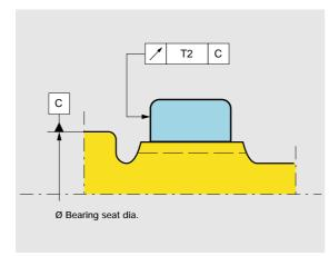
Whether the nut is threaded or pressed on, its clamping face must be perpendicular to the bearing seat. The axial run-out tolerance of the face is specified below.
