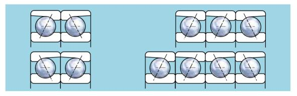
These arrangements can be made with universal bearings or sets matched by us at the factory. See characteristics of the different versions on page 24.
