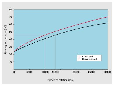
For an operating temperature of 45°C (113°F), the speed of rotation varies from 10,000 rpm with steel balls to 13,000 rpm with ceramic balls.
