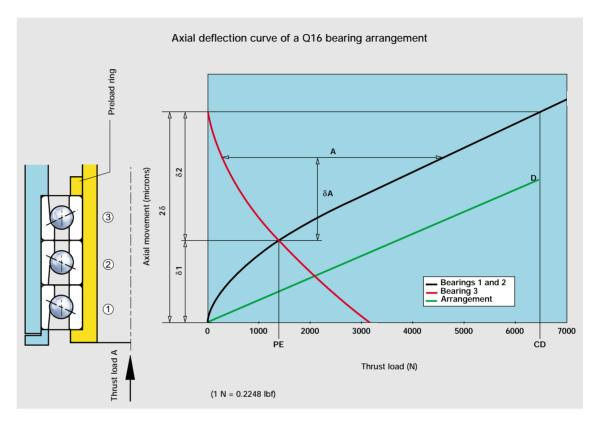
The thrust load A induces a displacement of the inner rings  $\delta A$ .
