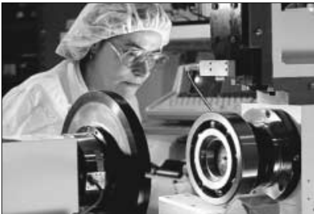
Barden’s Quiet Bearing Analyzer controls speed and load application to simulate “real world” operating conditions.
