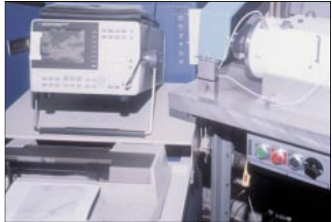
Barden's vibration test lab allows engineers to monitor and refine bearing performance in a spindle assembly under "real-world" operating conditions.
