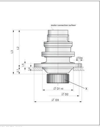
GFB T2/T3 2000 • X = The gearing of the output pinion (modul, number of teeth, tooth width, etc.) is governed by the customer's ring gear.
