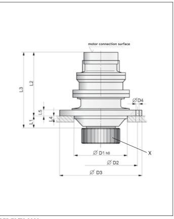
$GFB \ T2/T3 \ 2000 \quad \bullet \quad X = The gearing of the output pinion (modul, number of teeth, tooth width etc.) is governed by the customer's ring gear.$
