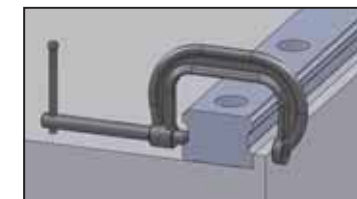
Fig 1.11.13 Mounting the master Linear Guide rail
